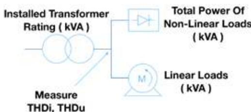
As said before the percentage of non-linear loads NLL is a very important indicator of magnitude of harmonics but a more detailed estimation of the magnitude of harmonics can be made with measurements.
