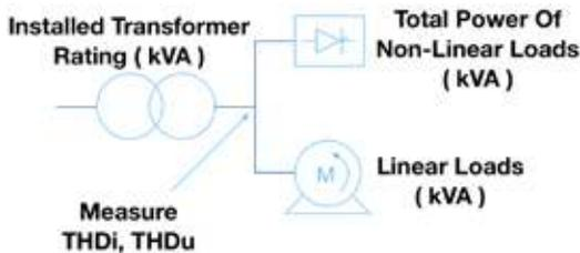
As said before the percentage of non-linear loads NLL is a very important indicator of magnitude of harmonics but a more detailed estimation of the magnitude of harmonics can be made with measurements.
